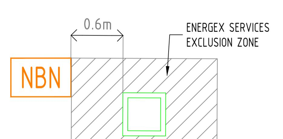
WHERE PITS ARE NOT LOCATED BESIDE PILLARS, OFFSETS WILL BE SHOWN ON THE LAYOUT TO THE NEAREST TRUNCATION. IF NO OFFSET DISTANCE IS SHOWN, PLEASE CONTACT DESIGN CONSULTANT PRIOR TO INSTALLATION.
